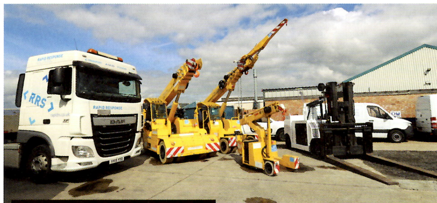
RRS runs DAF trucks, 2 to 18 tonne capacity Valla pick and carry cranes and 12 tonne capacity Hoist FR40/60 forklifts.
