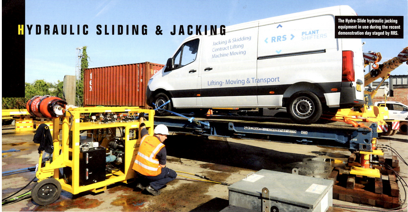
A Hydra-Pac synchronous power pack being used with the Hydra-Slide LP350 low profile skidding system.
