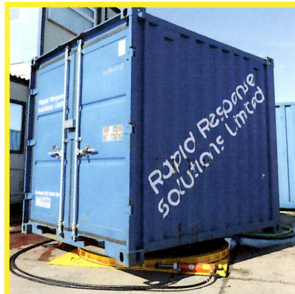
This 136 tonne capacity low profile TT150-6 hydraulic turntable was used to rotate a 10-foot container.
